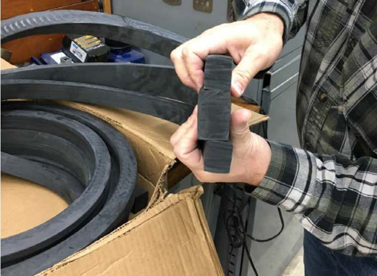
Photo 3. Example of square packing to be installed.
