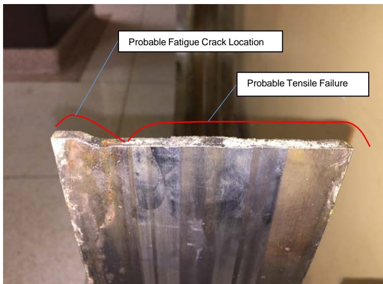
Photo 2. Fatigue on left side of sleeve after removal from unit 2.
